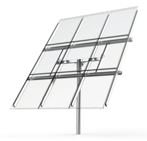
The Sentinel Solar Titan-TPM is a light-weight pole mounted module mounting system. The adjustable pitch between  $20^{\circ}$  and  $70^{\circ}$  allows for manual seasonal adjustment. It can hold up to  $9 \times 60$ -Cell, or  $6 \times 72$ -Cell PV Modules. The entire frame is mounted to a single 6'' Post.
